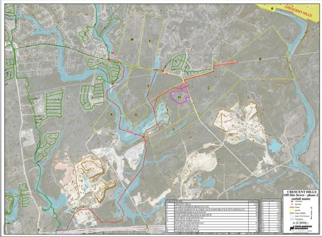
SAWS has determined that oversized mains are needed to <u>serve other developments</u> <u>anticipated to be built in this area</u>. <u>Sewage infrastructure was to be installed in creeks</u> that recharge the Edwards Aquifer.
