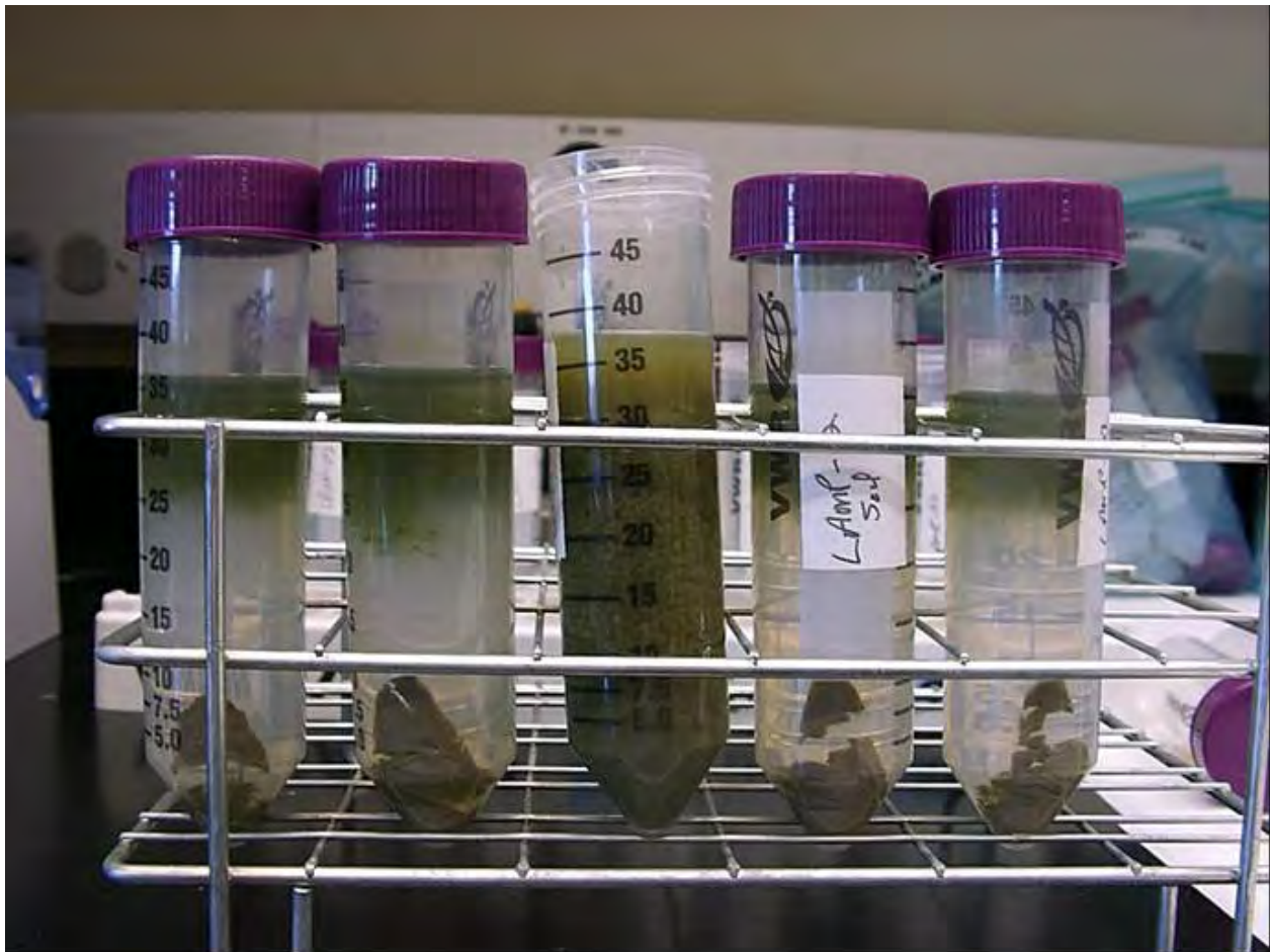
Figure 7. Photograph of a subsample of homogenized periphyton suspended in water (middle tube) following laboratory processing (bulk, or unfractionated periphyton), and four tubes containing aliquots of periphyton that were suspended in colloidal silica and centrifuged to separate the organic matter (algae, bacteria, detritus, fungi) from heavier, mostly inorganic particles (silt, clay, sand). The lighter organic material is pulled to the top of the suspension, whereas the sediment is pulled to the bottom during the centrifugation process. Following centrifugation, the organic fraction is removed using a pipettor, dried, pulverized, and analyzed for total carbon, nitrogen and phosphorus. The unfractionated bulk periphyton sample is dried, pulverized, and analyzed in the same manner but without separation from inorganic particles. See Appendix B for details.
