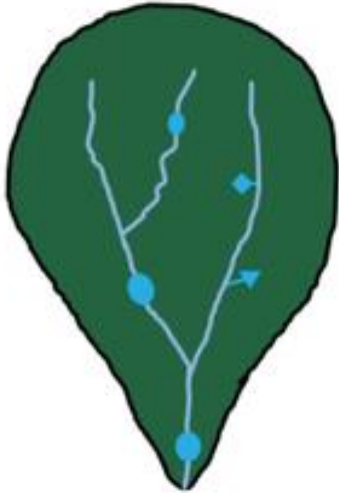
Conventional infrastructure with centralized stormwater facilities
