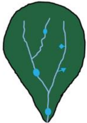
Conventional infrastructure with centralized stormwater facilities
