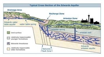
artesian zone is under pressure, causing water to be forced back to the surface as springs or wells. The <u>image</u> to the right illustrates the underground structure of the Edwards Aquifer.
