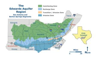
The Edwards Aquifer is a karst aquifer, meaning its underground structure is characterized by porous, permeable limestone that allows rainwater to quickly travel underground. The aquifer can be divided into three zones: the drainage area, the recharge zone, and the artesian zone. During and after
