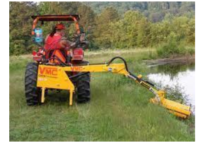
Figures 23 & 24: Extended boom mowers keep equipment out of wet areas
