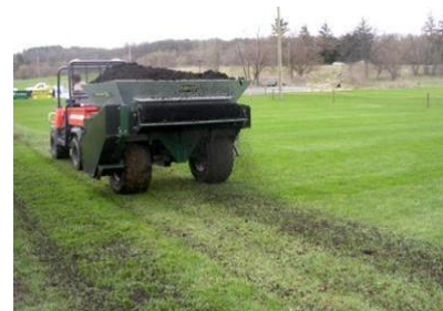
Figures 27 & 28: Soil amendment spreaders facilitate amending turf areas
