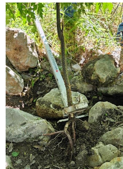
Figure 11: A weed wrench can be made or purchased in different sizes to remove larger tree seedlings.
