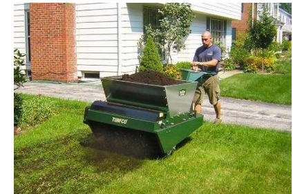
Figures 27 & 28: Soil amendment spreaders facilitate amending turf areas
