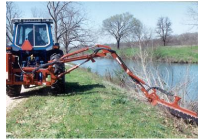
Figures 23 & 24: Extended boom mowers keep equipment out of wet areas
