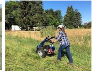
Figure 25 & 26: Sickle bar mowers for LIMA areas will allow the vegetation to be cut 6" or higher
