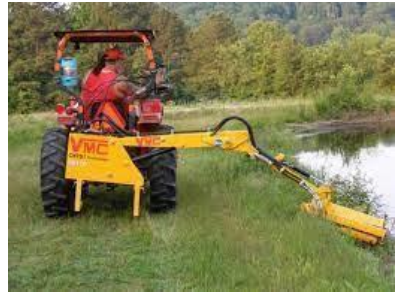
Figures 23 and 24: Extended boom mowers keep equipment out of wet areas.
