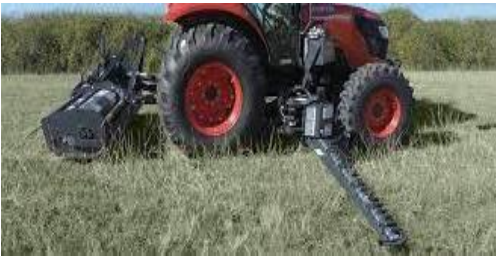
Figure 25 and 26: Sickle bar mowers for LIMA areas will allow the vegetation to be cut 6" or higher.
