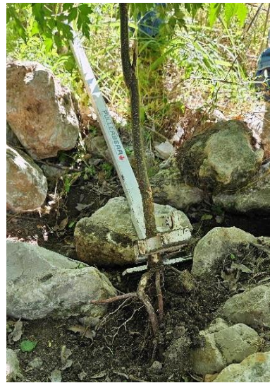
Figure 11: A weed wrench can be made or purchased in different sizes to remove larger tree seedlings.
