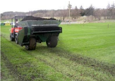
Figures 27 and 28: Soil amendment spreaders facilitate amending turf areas.
