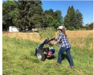
Figure 25 and 26: Sickle bar mowers for LIMA areas will allow the vegetation to be cut 6" or higher.
