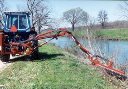
Figures 23 and 24: Extended boom mowers keep equipment out of wet areas.
