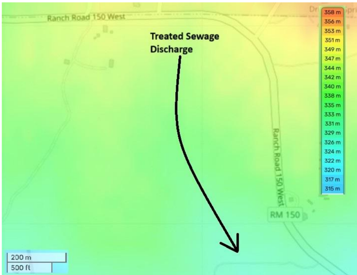
Fig. 2: The “unnamed tributary” proposed for receiving treated sewage discharge has little elevation change over its course, as shown in this topographic elevation map.
