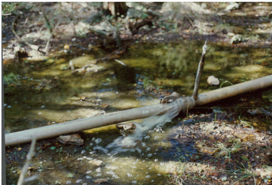
June 1989 photograph by Danny Brasher of Texas Water Commission of leaking wastewater irrigation line associated with Travis County wastewater disposal system
